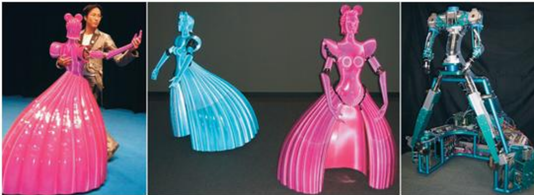
Figure 17 - The Dance Partner Robot. A force-torque sensor between the robot's upper and lower body measures the human leading force-moment. An omnidirectional mobile base uses special wheels to move along dance-step trajectories. (retrieved from [30]).
