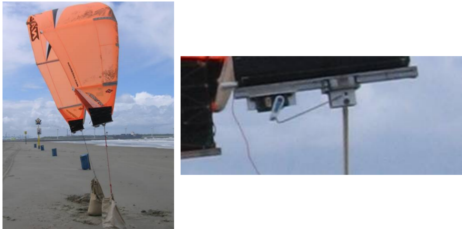
Figure 2.11: Slide mechanism on the kite [1].
