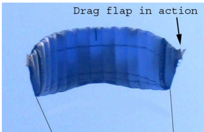
Figure 2.10: Drag flap control mechanism [8].
