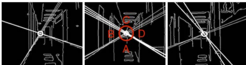
Figure 2.6: Hough Lines in the left and right wall
