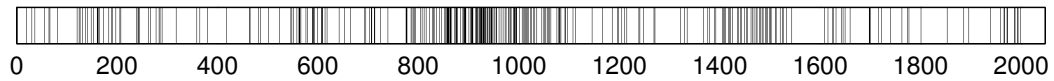
Figure 4.7: Bit error pattern upon the transmission of 2048 bits at the marina. Relevant parameters: two tones, 20 m distance, 375 symbols/s baud rate, 256 point DFT, an overlapp factor of 15/16 and 240 out of 255 transmission gain.
