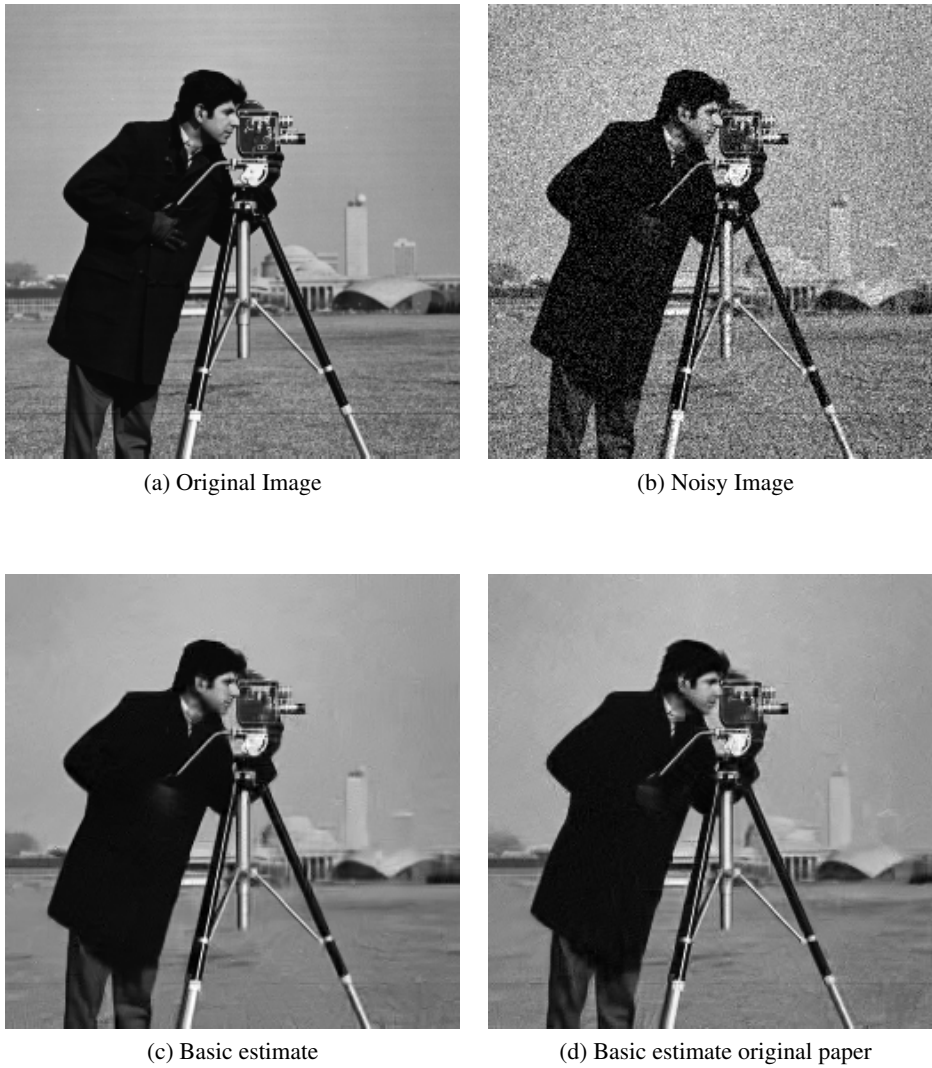
Figure 4.1: a) Original Cameraman image with size 256x256; b) Noisy image with \sigma = 25 (PSNR=20.17 dB); c) Basic estimate obtained by this implementation (PSNR=29.08 dB); d) Basic estimate of the original paper (PSNR=29.14 dB)
