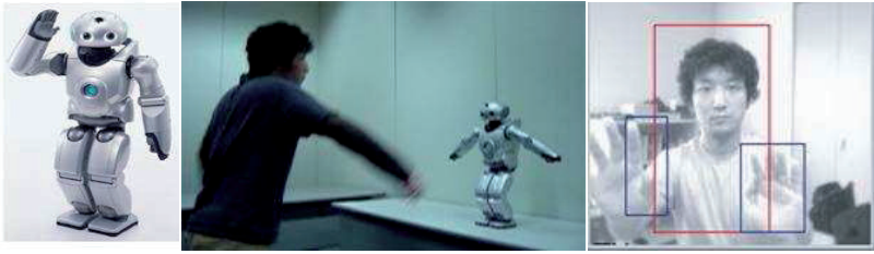
Figure 11 – Sony entertainment robot QRIO (Tanaka & Suzuki, 2004): a) QRIO humanoid robot [left]; b) QRIO reacting to human movement by following its rhythm and shape [middle]; c) A set of moving-regions obtained by QRIO's cameras [right].
