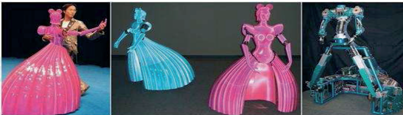
Figure 15 - The dance partner robot (Takeda, Hirata, & Kosuge, 2007): a ) A force-torque sensor between the robot's upper and lower body measures the human leading force-moment [left]; b ) MS DanceR two-colors layout [middle]; c ) An omni-directional mobile base uses special wheels to move along dance-step trajectories [right].
