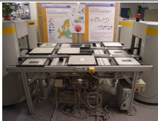
Fig. 3. FlexLink DAS 30 system (located at the Schneider Electric GmbH in Seligenstadt, Germany) [13]
