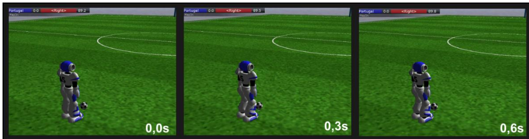
Figure 3.2. Following transfer of the robot to single support
