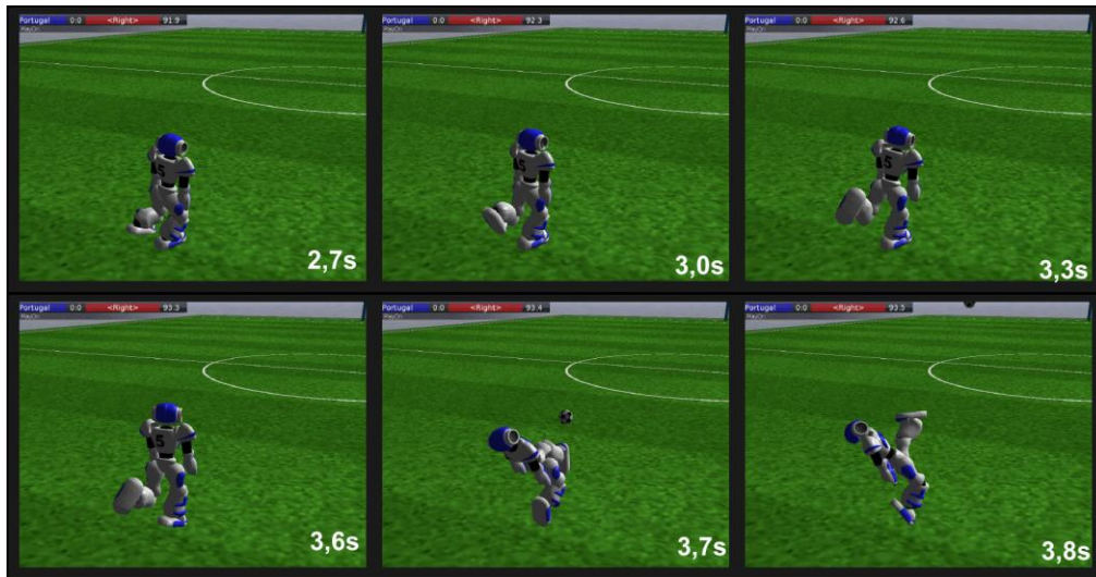
Figure 3.9. Sequence of the kick's poses placing and respective kick
