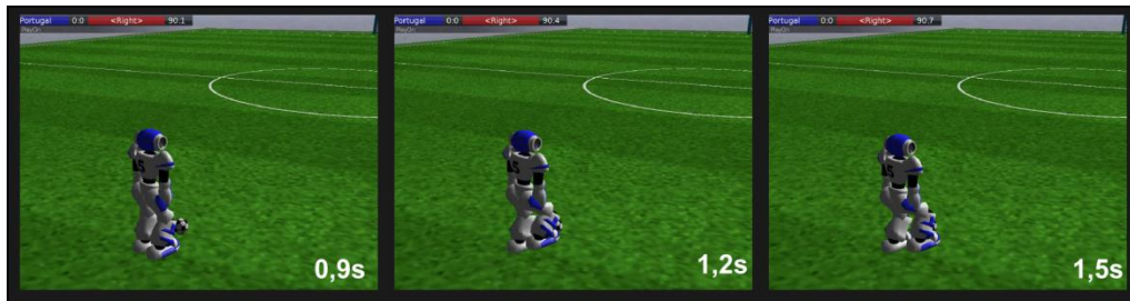
Figure 3.5. Sequence of the lowering and placing support foot
