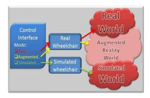
Figure 5: Intelligent Wheelchair Platform Architecture.
