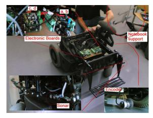
Figure 3: Devices installed in IW.
