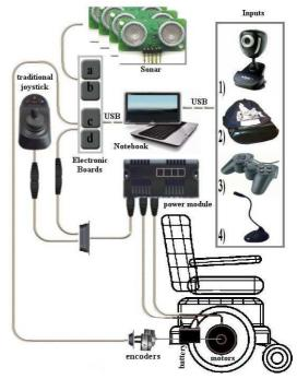
Figure 1: Hardware Architecture of IntellWheels.
