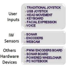
Figure 2: Hardware Functional Blocks.
