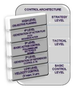
Figure 6: Control architecture.
