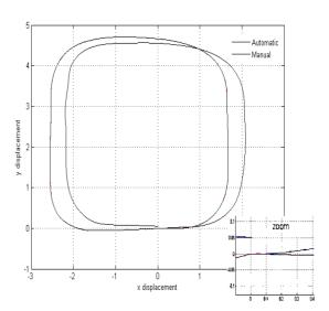
Figure 9: Path Followed by Wheelchair in the Tests.
