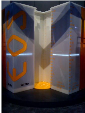
FIGURE 2.7: The EOS™ system from BioSpace Med, France. This system is able of capturing frontal and lateral radiographs of the patient simultaneously.
