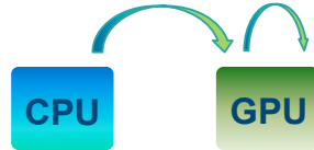
Kepler: GPU can generate work for itself.
