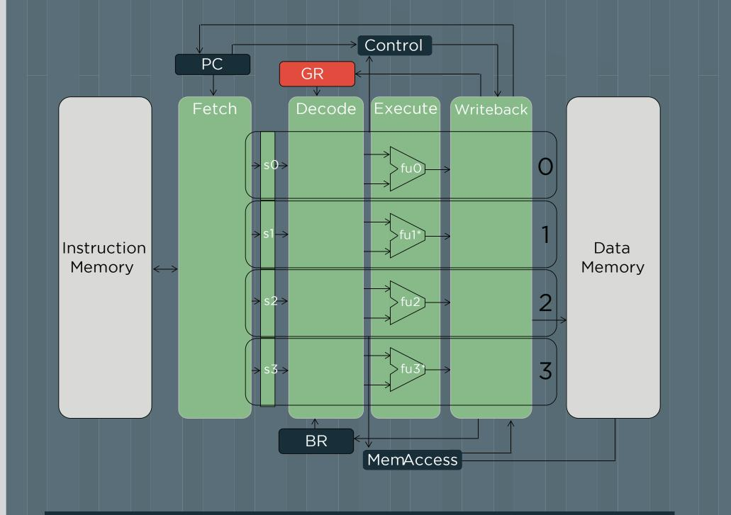
The p-Vex is a configurable and extensible VLIW processor, based on the VEX ISA, that supports multiple issue widths. We have used the 4-issue version of this architecture
