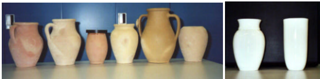
Figure 2 - Pots used in laboratory measurements (left: pots 1 to 6 of unglazed terra-cotta, right: pots 7 and 8 varnished)
