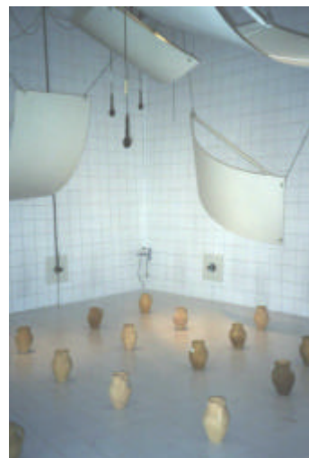
Figure 3 - (left) Measurements in anechoic room with an enclosed pot Figure 4 - (right) Measurements in reverberant chamber with 30 scattered pots
