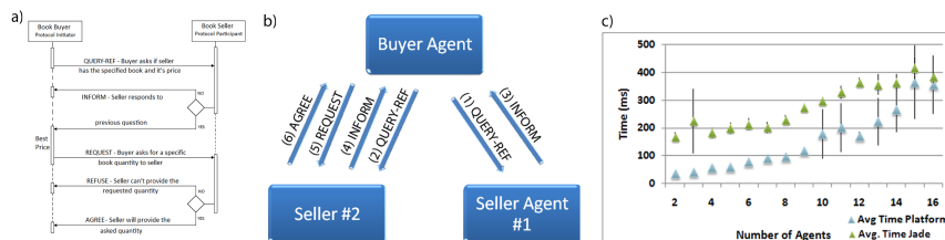
Fig. 4. Book buyer and book seller agents' protocol, a). An example of message exchange in this test scenario with seller #2 providing the book's best price, b). Test's results for Jade and the described platform, c).
