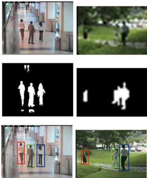
Figure 2: Segmentation results (second row) using the cascaded change detection algorithm and tracking results (third row) using the Kalman filtering with appearance constraints.
