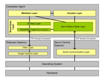
Fig. 4. Catrapilas Architecture
