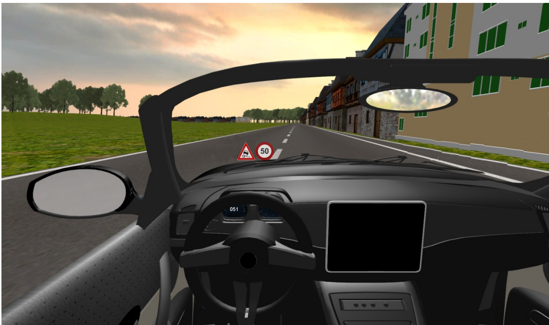
Figure 22: Example of a situation where both warnings are activated. Warnings are projected onto the windshield.
