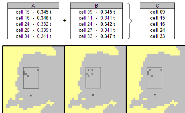
Fig. 3. FarmerGA breeding result: A and B - parent configurations; C - child configuration
