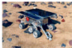
Rocky 7, with stereo vision and sampling manipulator
