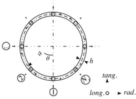
Figure 3. Cross-section of a thin-shell divided into  $N_s$  nodes.
