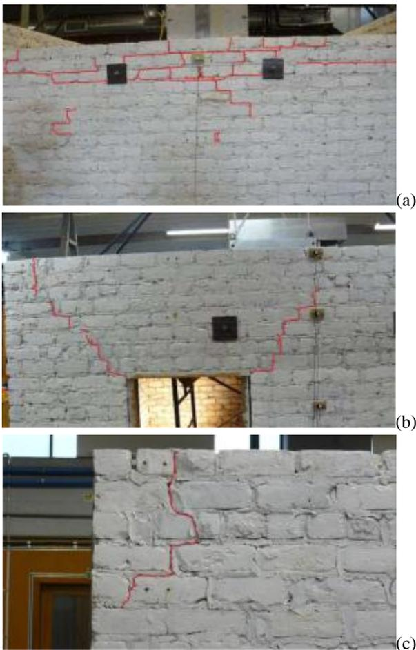
Figure 4. Damage observed at DS3. (a) South wall, (b) North wall, and (c) North-west walls' corner
