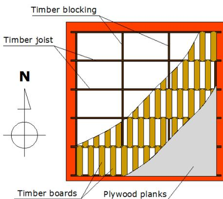
Figure 2. Timber diaphragm layout.
