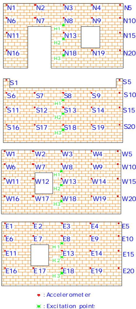
Figure 6. Measurement grid and excitation points. (a) North wall, (b) South wall, (c) West wall, and (d) East wall
