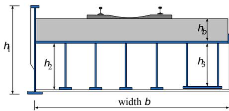
Figure 2. Cross-section of the elaborated 3D-FE bridge.
