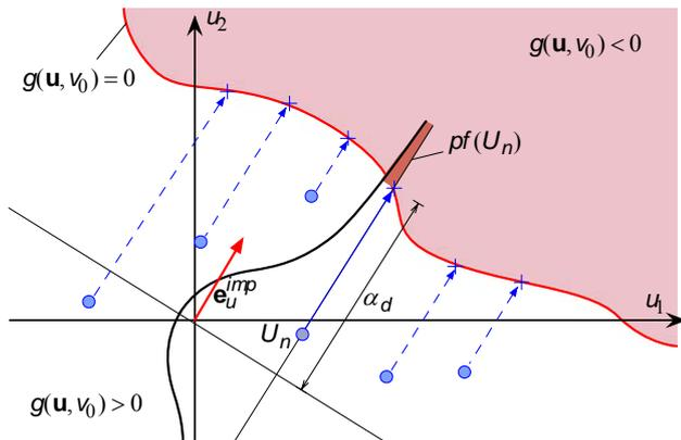
Figure 5. LS procedure in standard normal space.
