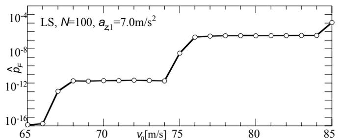
Figure 11. Estimates of the probability of failure for increasing design speed  $v_0$ .
