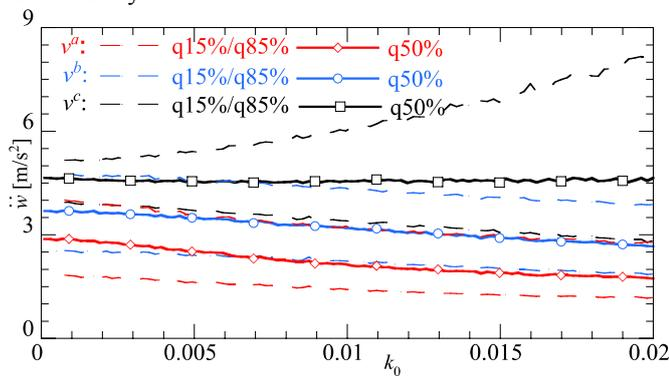
Figure 12. Maximum acceleration at speeds  $v^a$ ,  $v^b$ , and  $v^c$ . Linear temperature-frequency relation,  $k_1 = k_0$ .
