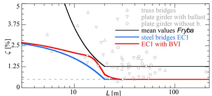
Figure 3. Modal damping coefficients  $\zeta$  for steel bridges according to [2] and [6].
