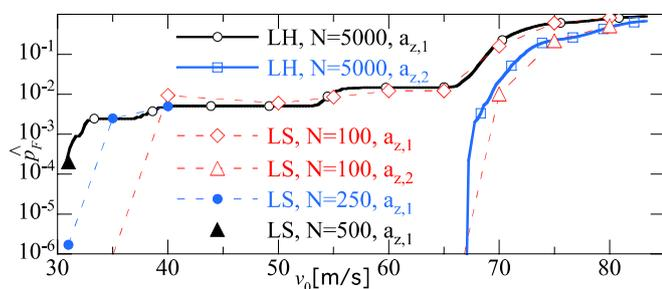
Figure 19. Estimates of the probability of failure for increasing design speed  $v_0$ , elaborated bridge model.
