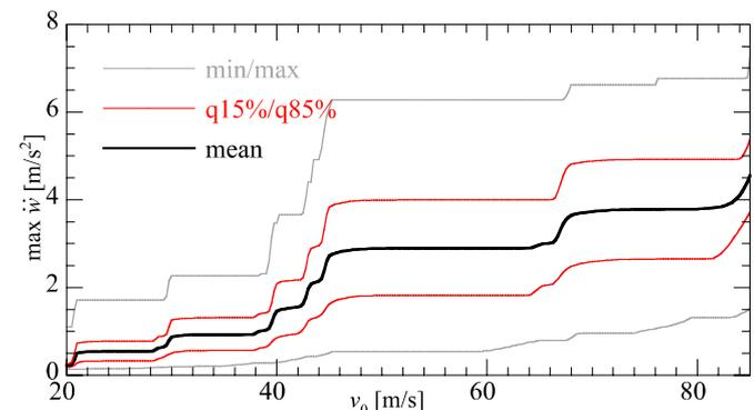
Figure 8. Spectrum of maximum acceleration of the beam bridge subjected to the HSLM-A train set with respect to the design speed  $v_0$ .
