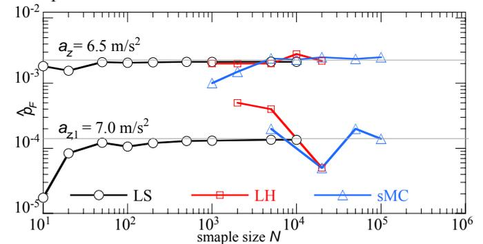
Figure 9. Estimates of the probability of failure for different simulation methods, sample sizes and limit states.
