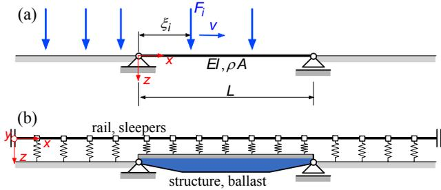
Figure 1. Mechanical bridge models: (a) *Bernoulli-Euler* beam bridge and (b) elaborated 3D-FE bridge (side view).
