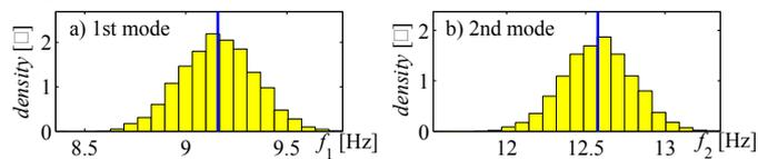
Figure 15. Distribution of the natural frequencies of the first and second mode.
