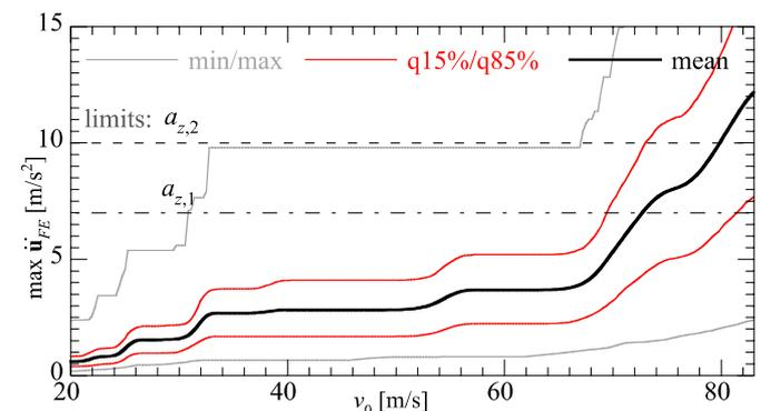
Figure 18. Spectrum of maximum acceleration induced by HSLM-A train set for design speed  $v_0$ , elaborated bridge model.
