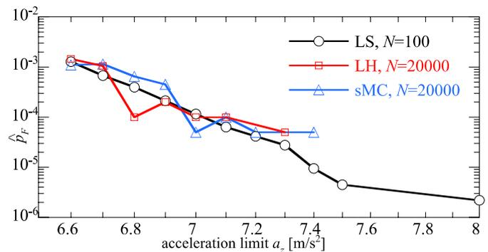
Figure 10. Estimates of the probability of failure for increasing acceleration limits.
