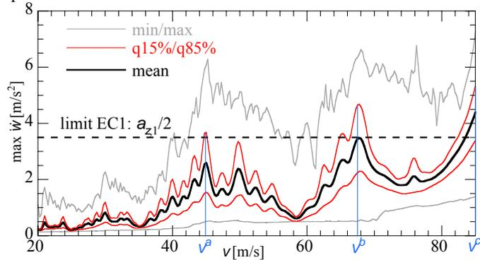
Figure 7. Spectrum of maximum acceleration of the beam bridge subjected to the HSLM-A train set with respect to the actual train speed  $v$ .
