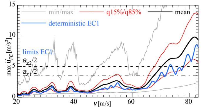
Figure 17. Spectrum of maximum acceleration induced by the HSLM-A train set for actual train speed  $v$ , elaborated bridge model.
