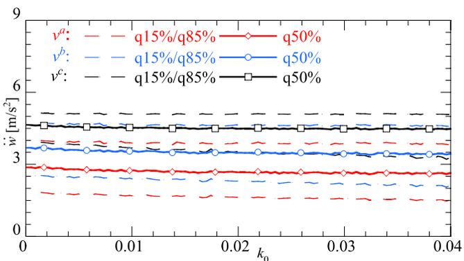
Figure 13. Maximum acceleration at speeds  $v^a$ ,  $v^b$ , and  $v^c$ . Bilinear temperature-frequency relation,  $k_1 = 0.001$ .
