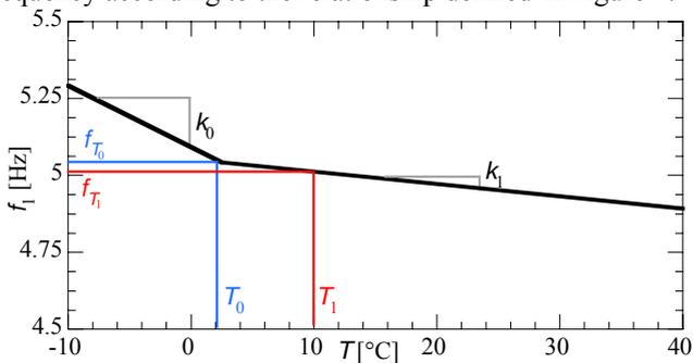
Figure 4. Bilinear relationship between the fundamental natural frequency and the environmental temperature.
