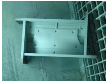
Fig. 6 - Half mould after deposition of the metallic coating.
