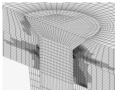
Figure 2: Distortional strain invariant index around a loaded single lap bolted joint including the effect of bolt clamp-up. (Darker tone represents a higher index)
