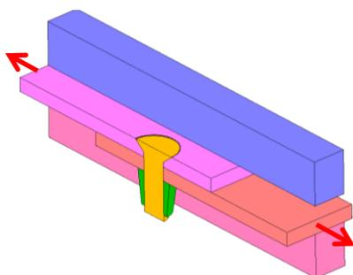
Figure 1: Geometry of single lap countersunk bolted joint model including the ATSM D 5961 test fixture and the direction of the applied displacements.
