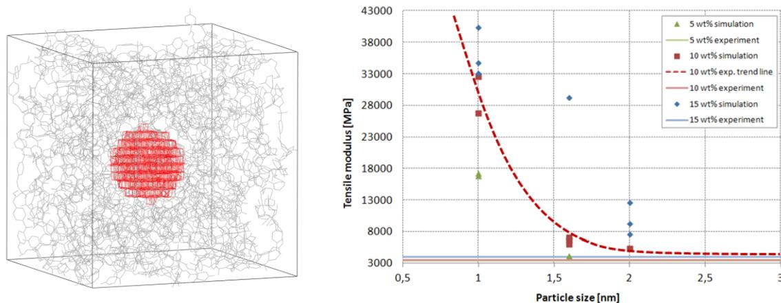
Figure 1: 2 nm particle 15 wt%, (left) tensile modulus for various weight fractions (right)
