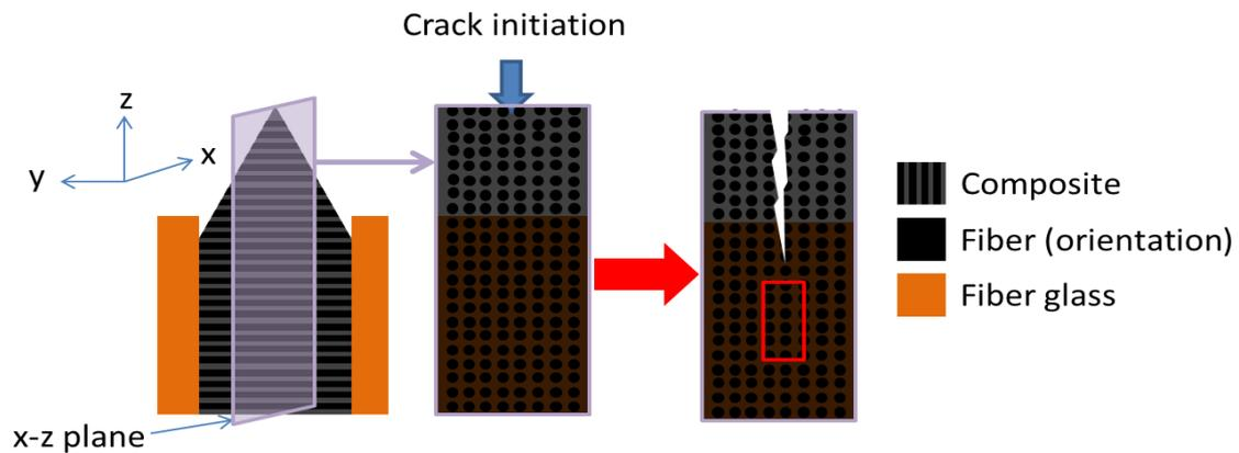
Fig. 1 Specimen configuration for crack arrest.
