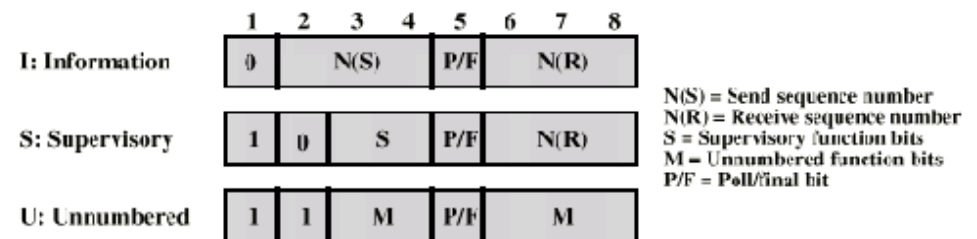
8-bit control field format
