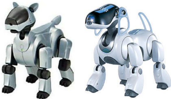
Figure 1: ERS210A (left) and ERS7 (right) AIBO Sony quadruped robotic platforms.
