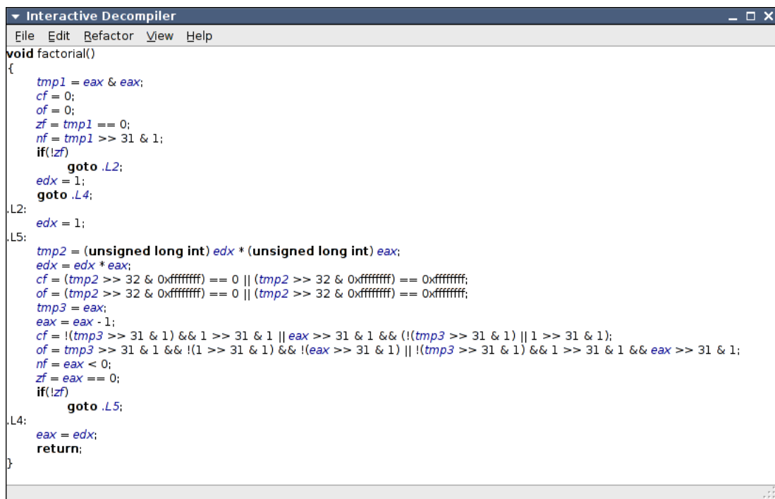
Figure 5.6: Code after applying the Extract Function refactoring
