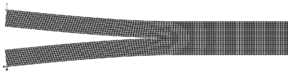
Fig. 4 – Mesh used in the DCB simulation.
