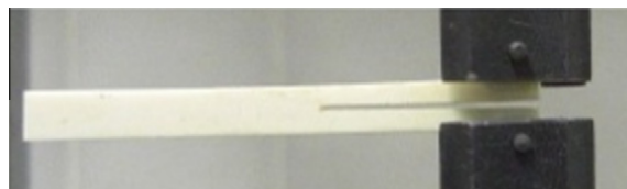
Fig. 4. Photography of the DCB test.
