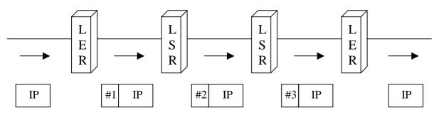
Figure 2 – Label insertion, swapping and removal
