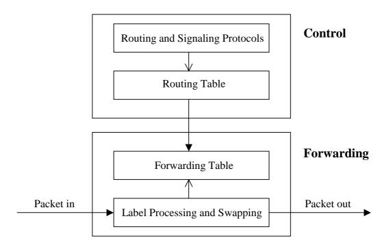
Figure 1 – Mapping between routing and forwarding tables
