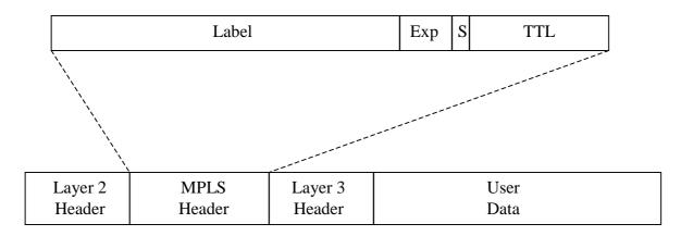
Figure 3 – MPLS header and encapsulation
