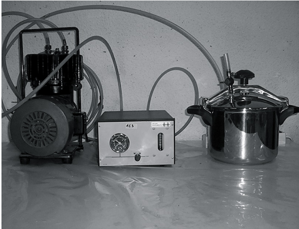
Figure 9: Vacuum impregnation assembly. Pump, control of the pump and pressure cooker
