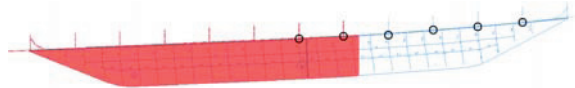
Figure 5. Valid domain for the design load, overlapped with the location of the recorded cracks.
