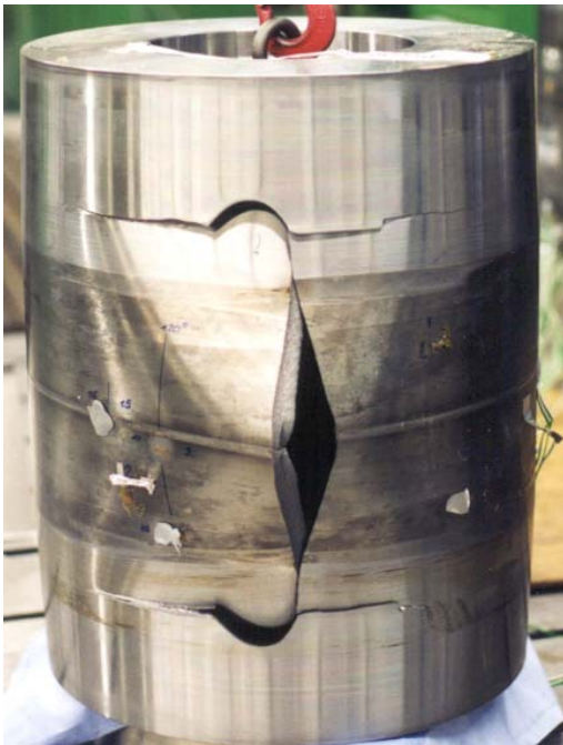
Figure 8: Sub-Scale Pressure Vessel after Burst Test
