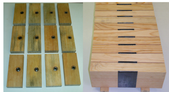
Figure 1. Specimens reinforced with metallic inserts (left) and CFRP laminates (right).
