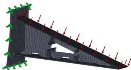
Figure 6. Three-dimensional model of the bilge keel section modeled, which includes the internal structural arrangement, the finite element mesh, the design load and the boundary conditions.
