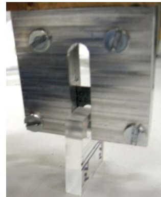
Figure 6. Razor blade support device and application into CT-fracture specimen.
