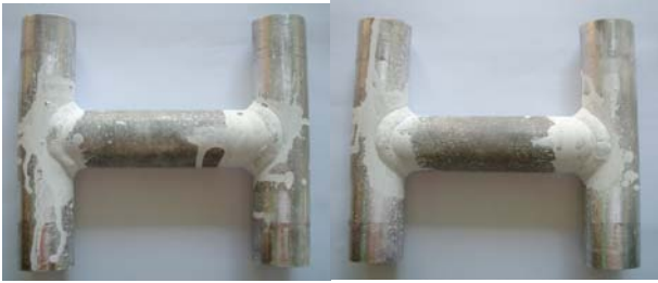
Figure 13. Liquid Penetrant Testing.
