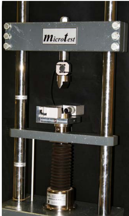
Figure 1. Test machine MICROTTEST EM1/50 with the experimental set up.
