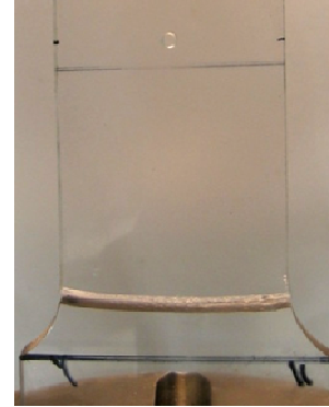
Figure 9. Plate with 3 mm diameter hole, after rupture near the filleted zone (and not at the hole).
