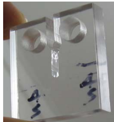
Figure 8. CT-fracture specimen with a successfully obtained natural crack.
