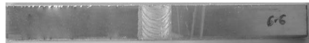
Figure 3. Photo of a fatigue specimen cut from welded plate before edges machining.
