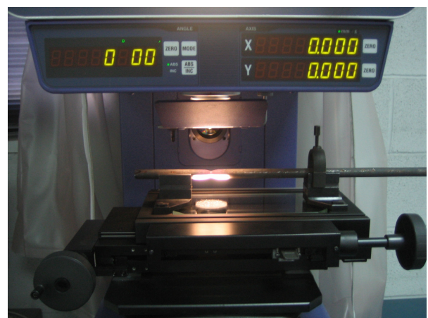
Fig.3.- Arrangement of the sample on the profile projector.
