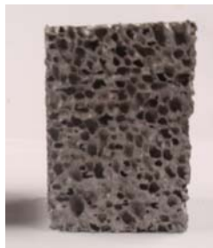
Figure 2. Alporas specimen for quasi-static compression ( \rho^*/\rho_s = 0.1 ).
