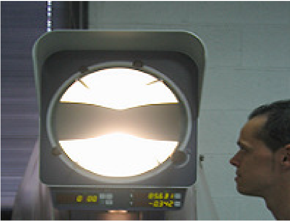
Fig.4.- Profile projector screen where the formation of necking in the sample may be observed after the tensile test. The neck diameter is measured on this screen.
