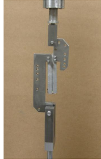
Figure 2. Fixtures with the MCB-specimen.
