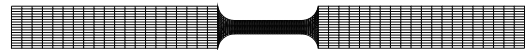
Figure 6. Finite element mesh for the plane strain specimen with 1600 elements and 5033 nodes.
