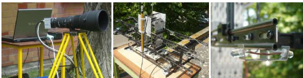
Figure 5 - experimental test: (left) the camera C_1 mounted in the tripe; (centre) the targets structure and displacement transducers mounted in the platform; (right) detail of the LED support, where the target is represented by a pair of LEDs.
