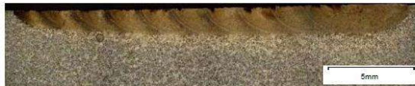
Figure 2 – OM images of overlapped melt tracks from LSM samples.
