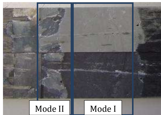
Figure 3 – Fracture surfaces of the specimens tested with 50% of the load.
