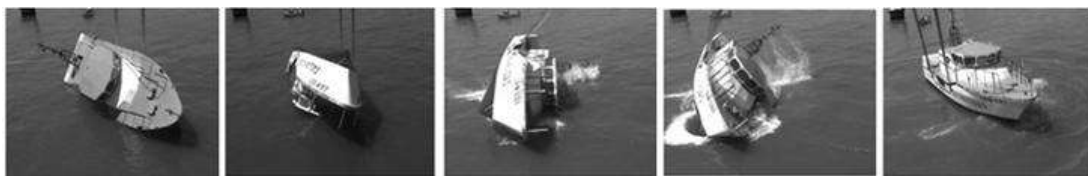
Figure 1 - Self-righting ability of the HSLC under study, that was designed, fabricated and is successfully operating in Portugal
