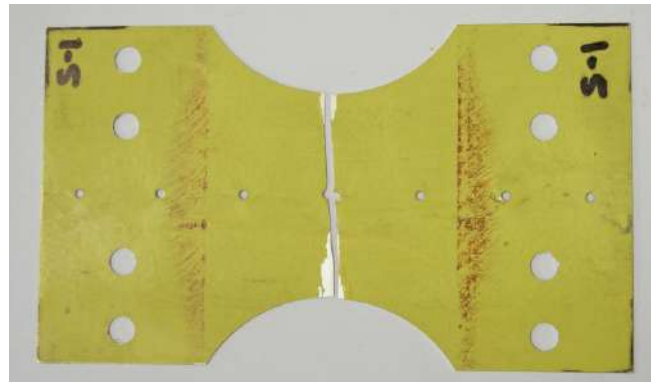
Figure 4 - Fatigue cracking from a rivet hole in a coupon
