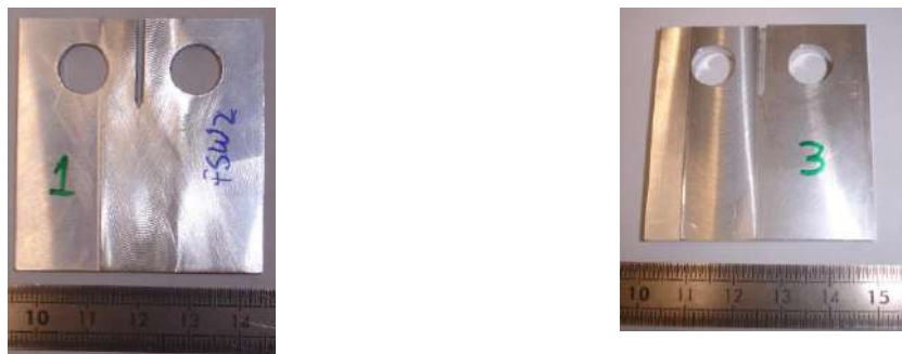
Figure – example of specimens tested, with crack in the nugget (left) and in the HAZ (right)
