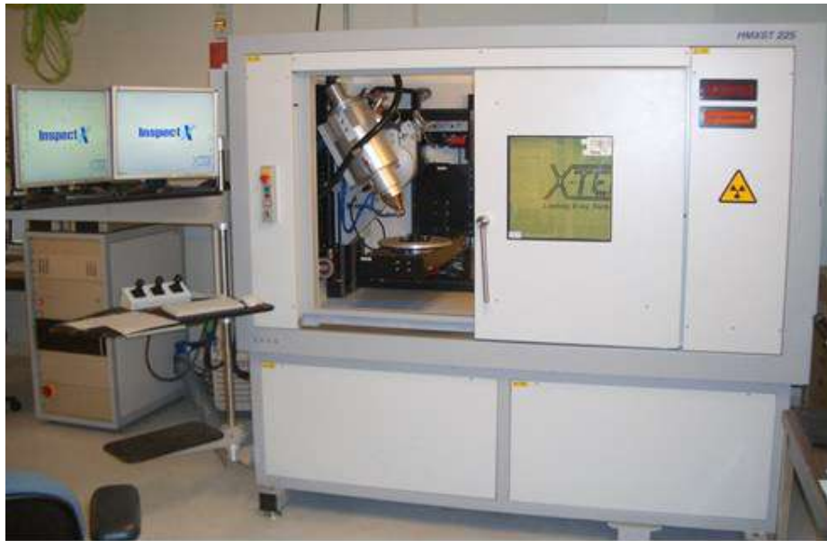
Figure 5 - XTEK tomography equipment with X-Ray source.
