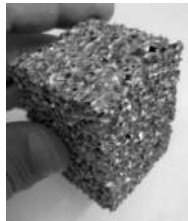
Figure 3 - Aluminium metal foam (Alporas foam \bar{\rho} = 9\% ).
