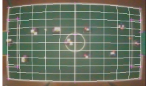
Figure 3. Correction of the barrel distortion
