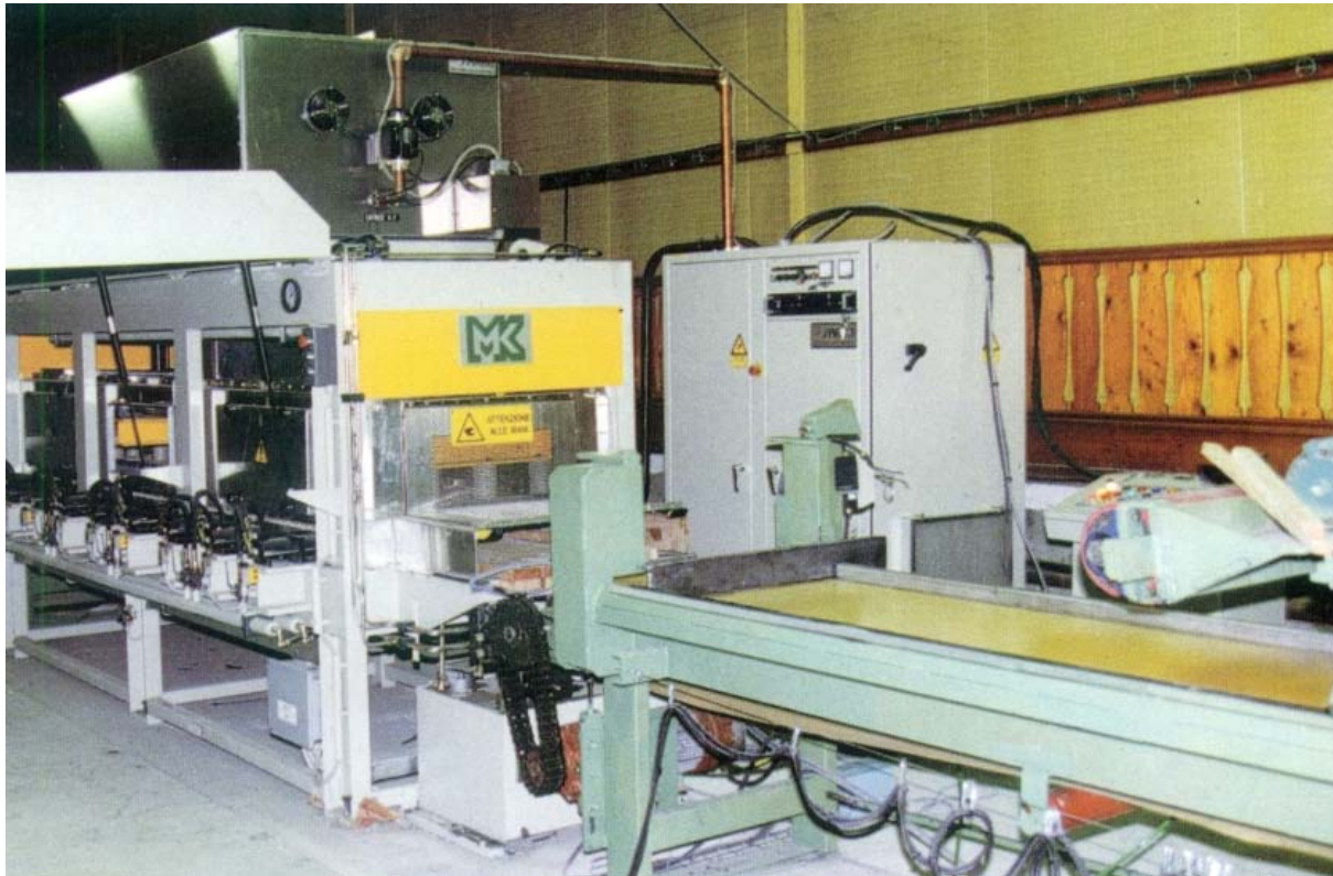
HF heating machine (SAIREM) at CTBA
