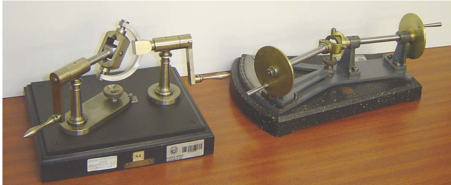
Fig. 2 - Cardano's coupling by Voigt (left) and by Schröder (right), belonging to FEUP
