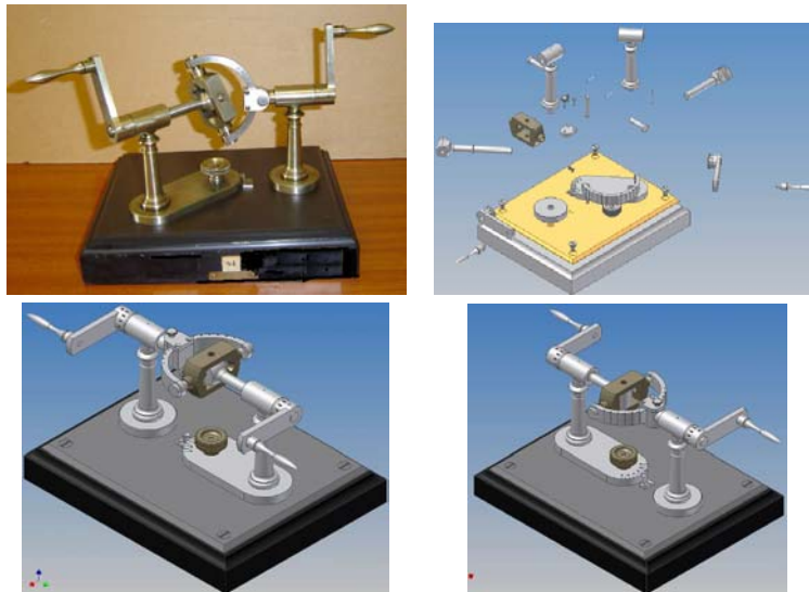
Fig. 6 - Modelling of the Voigt model of the Cardano's Coupling [17]
