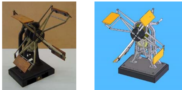
Fig. 7 - Modelling of the Four Paddle Wheel Propeller [18]
