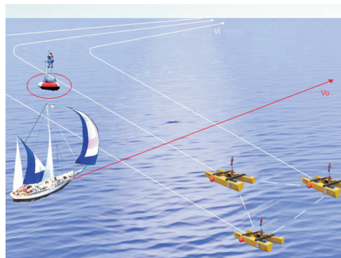
Fig. 1. Collision avoidance: a group of autonomous surface craft on a data-gathering mission at sea.
