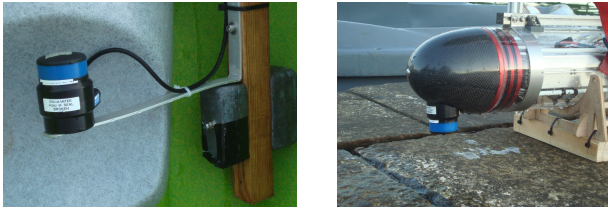
Fig. 4. Fixed transponder (left) and acoustic modem on the Medusa nose cone (right).
