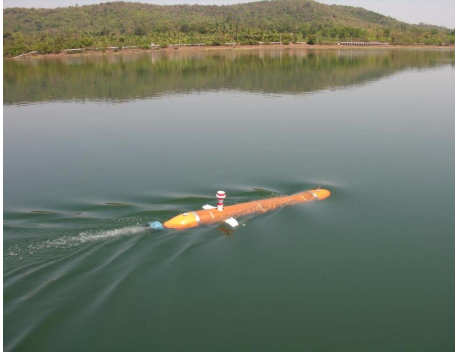
Fig. 7. The MAYA AUV
