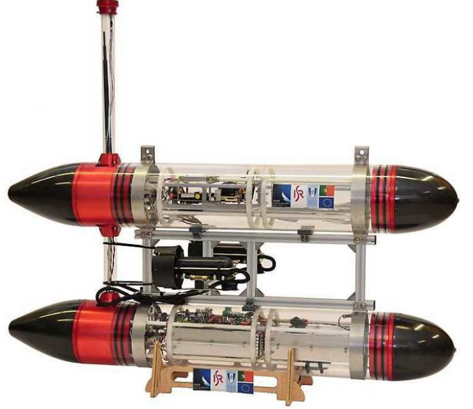
Fig. 1. The MEDUSA vessel set-up. The thrusters are mounted in the middle between both hull parts on the x - z -plane (body coordinates) and produce completely from the body on the x - y -plane.
