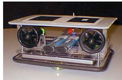
Fig. 1. The MVWT vehicle. A laptop is secured in a Plexiglas chassis that glides on omnidirectional ball casters. Software-controlled high-powered ducted fans attached to the vehicle provide thrust. A MVWT signature on the top the vehicle ( a “hat”) is identified by overhead cameras, and the vehicle receives its position and orientation in a GPS-like fashion over a local wireless network.
