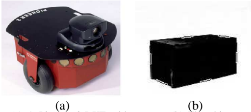
Fig. 1. (a) A Pioneer 2-DXE with camera. (b) The object seen by the camera used for calibration.
