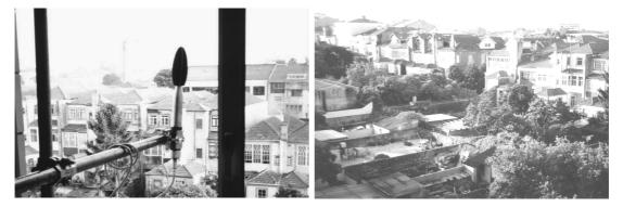
Figures 1 & 2. Outdoor microphone installation and sight of the measured backyard
