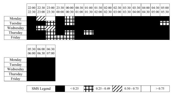
Figure 6. SMS variation in four groups of values within pre-defined time intervals - nighttime period (allowable error  $\pm 0.5$  dB(A))
