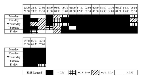
Figure 7. SMS variation in four groups of values within pre-defined time intervals - nighttime period (allowable error of  $\pm 1.0$  dB(A))
