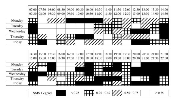
Figure 5. SMS variation in four groups of values within pre-defined time intervals - daytime period (allowable error  $\pm$  0.5 dB(A))
