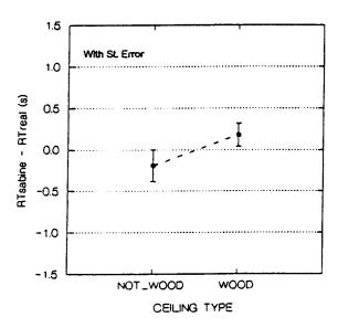
Fig. 4 - Analysis of the effect of ceiling type (wood and non wood) differences ( $RT_{REAL} - RT_{SABINE}$ ). Mean values for all the churches in each ceiling type are shown with one stand. error confidence interval.
