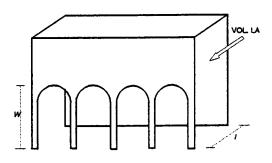
Fig. 2 - 3-D sketch of lateral aisles in a general church. *l*-width of lateral aisle, *w*-width of opening to lateral aisle, vol<sub>LA</sub>-volume of lateral aisle.
