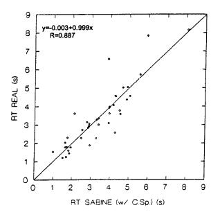
Fig. 3 - Plot of measured ( $y \ axis$ ) vs. predicted ( $x \ axis$ ) RTs with linear prediction line and Pearson correlation coefficient.
