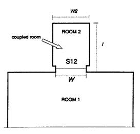
Fig. 1 - Plan sketch of a general church with a coupled space. *l*-length,  $S_{12}$ -opening surface area, *w*-opening width, *w*2-coupled space width, Room 1-main room, Room 2-coupled room.
