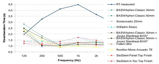
Figure 9: Measured and predicted RT in Room 11 (CAMS) for the suggested acoustical corrections.<sup>2</sup>
