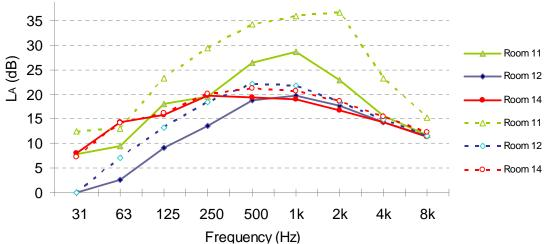
Figure 8: Background sound pressure levels (A weighted), with (-) and without (---) HVAC at CAMS.<sup>2</sup>
