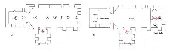
FIGURE 2: (A) Recording locations (1-8) on the nave floor for the impulse response tests and the source location (MA) on the nave floor.
