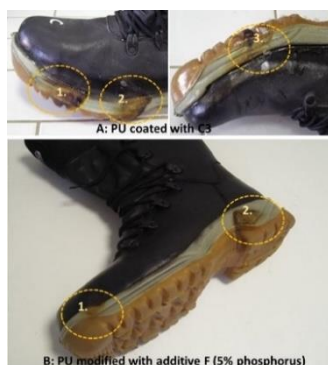
Figure 2. Prototypes produced following the two developed strategies, after flame resistant testing.
