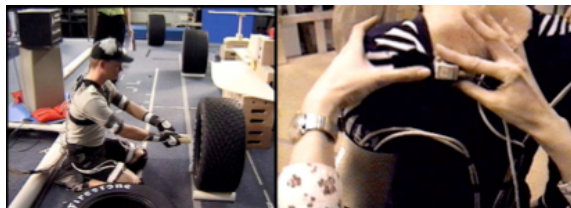
Figure 2: Left: Actor using magnetic mocap suit. Right: Close-up of a magnetic mocap sensor.
