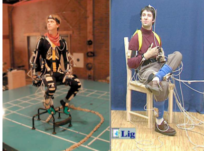
Figure 1: Left: Actor using full mechanical motion capture suit. Right: Actor using just some mechanical sensors instead of a full suit.
